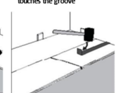
Step 8: Use hammer and pull bar to engage final piece, insert spacers and continue to next row.
